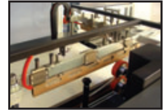
Vertical seal head with one piece seal knife and blade 2 yr warranty on seal blade
